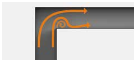
Angular pipe elbow: not flow-enhancing
