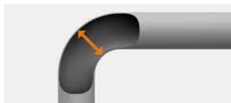
Round pipe elbow: flow-enhancing
