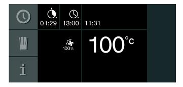
During the last minute of the cooking time the remaining time is displayed in an enlarged format.
