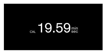
**Note:** Do not interrupt calibration. Do not turn the function selector. Do not open the appliance door.
