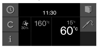
5 The appliance heats with the set heating mode. The current core temperature is displayed and, under it, the set core temperature. You can change the set core temperatur at any time.
