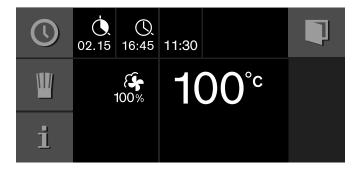
The appliance switches to standby. The heating mode, temperature, cooking time and cooking time end appear in the display. The appliance starts at the calculated time and switches off automatically when the cooking time has elapsed.
