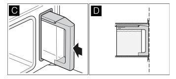
The tank must be flush with the water tank recess (fig. D).
