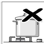
Always centre the pan over the burner, not to one side. Otherwise it could tip over.
