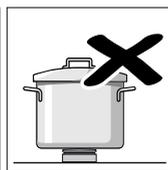
Place the pans on the pan supports, never directly on the burner.
