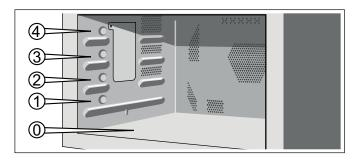
**Note:** Microwaveable ovenware can be placed on the oven floor (level 0).
