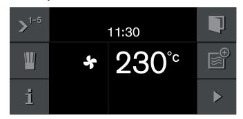
Depending on the operation mode selected, the symbol for microwave or the symbol for oven appears in the right-hand control panel, which enables you to add the other relevant operation mode.
