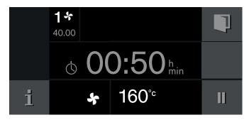
The appliance goes into standby mode. The display shows the operating mode, the temperature, the cooking time and the remaining time until the start. The appliance starts at the calculated time and automatically switches off once the cooking time has elapsed.
