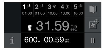
**Note:** You can set the temperature, grill setting for a type of oven heating and the cooking time for a microwave output using the rotary selector while the recipe is in progress. This does not change the saved recipe.
