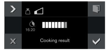
4 Confirm with ✓. The display switches to the programme. The cooking time is changed accordingly.
