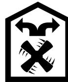
The air which is drawn in is cleaned by the grease filters and an activated carbon filter, and is conveyed back into the kitchen.
