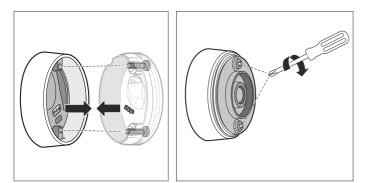
4 Put the silicone cover back on the lower section of the temperature sensor casing.
