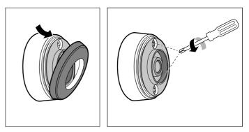
2 Remove the upper section of the casing. Remove the old battery. Insert the new battery. Make sure that the polarity is correct.
