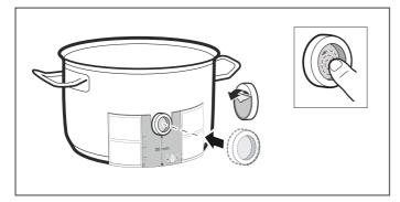
**3** Press the silicone patch down, and press on its inside surface too.
