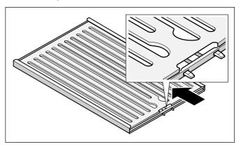
2 Push the metal mesh filter in completely.
