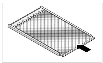
With the lock facing towards the front, place the metal grease filter in the underside of the appliance and engage the lock.
