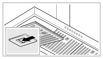
2 Slightly lift the front edge of the metal grease filter until it can be removed from the holder.
