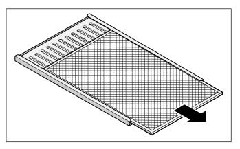
4 Pull the two parts of the filter apart, using the recessed grip to help you do this.
