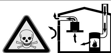
Room air-dependent heat-producing appliances (e.g. gas, oil, wood or coal-operated heaters, continuous flow heaters or water heaters) obtain combustion air from the room in which they are installed and discharge the exhaust gases into the open air through an exhaust gas system (e.g. a chimney).
