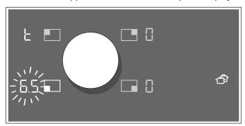
3 Select the new hotplate within 90 seconds using the twist knob. The settings have been transferred.
