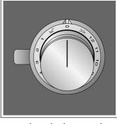
You can use the control knobs to select the heat setting, the PowerBoost function, the FlexZone and the wok function.
