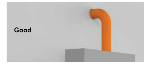
Any narrowing of the cross-section should be avoided
