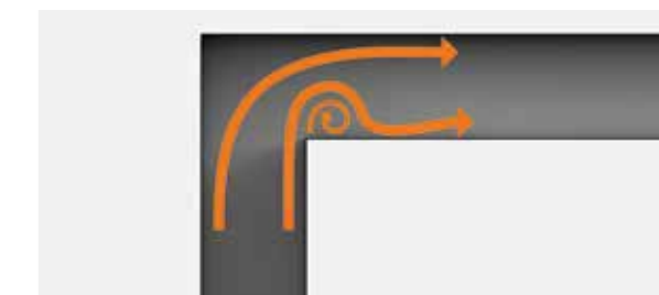
Angular pipe elbow: not flow-enhancing
