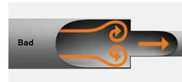
Any narrowing of the cross-section should be avoided
