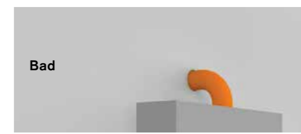
The section of the pipe downstream of the air outlet should be at least 30 cm long
