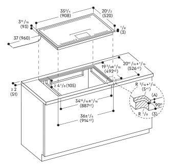
Minimum countertop thickness  $1^3/_{16}$ " (30 mm) for flush installation.
