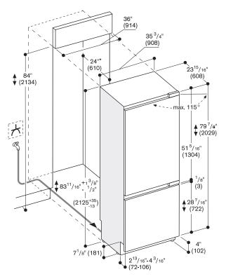
The door face dimensions are designed for a maximum gap of  $\mbox{1/8}\mbox{"}$  (3 mm).
