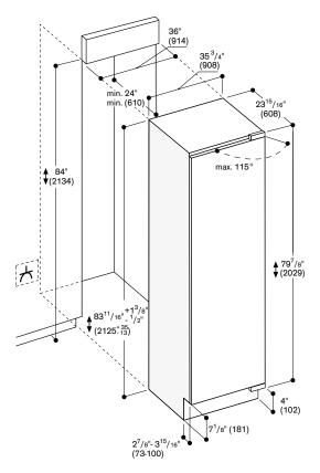
The door face dimensions are designed for a maximum gap of 1/8" (3 mm).
