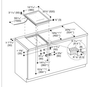
Minimum countertop thickness 1 3/16" (30 mm) for flush installation.
