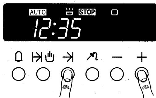
Four seconds after programming, the time of day is displayed again. The programmed switch-off time can only be queried by pressing the appropriate key.
