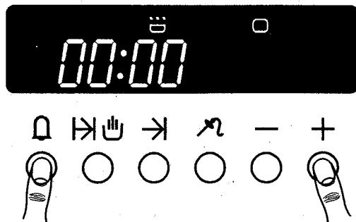
Press the "Short time **13**" key and keep it pressed. A suggested time of 00:00 appears in the timer display. Then press the PLUS key **17** to program the required time.
