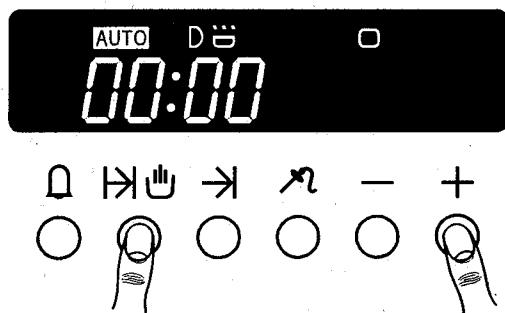
Four seconds after programming, the time of day is displayed again. The programmed duration can only be queried by pressing the appropriate key.
