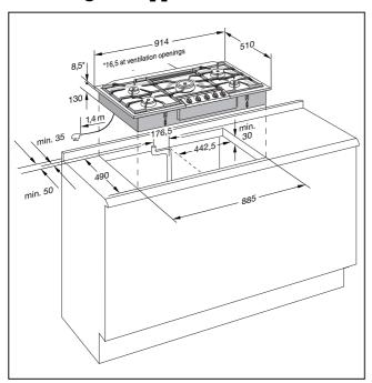
**Note:** the appliance can be installed in a base cabinet with a minimum width of 900 mm. The recess in the countertop will be slightly wider than the inner width of the base cabinet. Do not install the appliance above a drawer.
