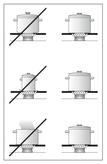
Pots with a diameter of less than **90 mm** or more than **280 mm / 320 mm for the large (WOK) burner** should not be used. When using large pots, pay attention to keeping to a minimum distance of **50 mm** between the cooking vessel and combustible surroundings.
