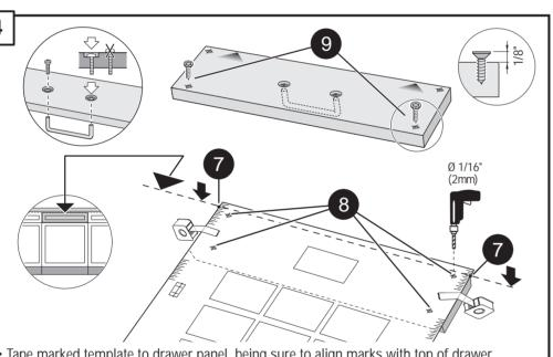
• Tape marked template to drawer panel, being sure to align marks with top of drawer. Then using drill start holes for brackets. DO NOT drill completely through drawer. • French blind text- French text- French blind text-French blind text- French-French blind text blind text- French blind text-French blind text- French-French blind text-
