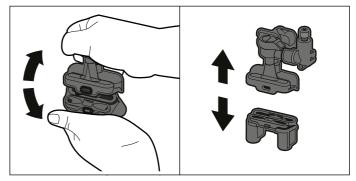
4 Separate the milk hoses, connecting element and milk tube.
