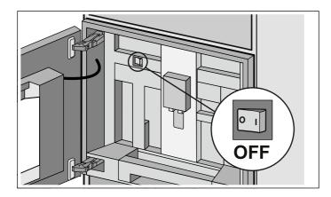
The main switch is used to switch the appliance on and off.
