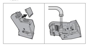
10 Remove the cover and clean the filter under running water.
