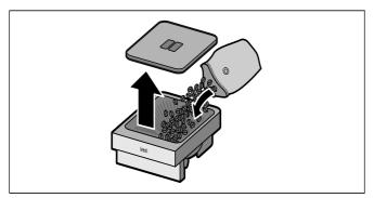
**Note:** Coffee beans that have been glazed or caramelised or that contain other sugary additives block the brewing unit. Only use pure bean mixes that are suitable for use in fully automatic espresso or coffee machines.
