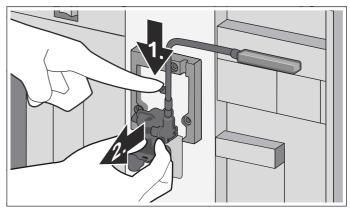
3 Detach the milk hose and dismantle the top and bottom sections of the beverage dispenser.
