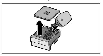
**Note:** Coffee beans that have been glazed or caramelised or that contain other sugary additives block the brewing unit. Only use pure bean mixes that are suitable for use in fully automatic espresso or coffee machines.
