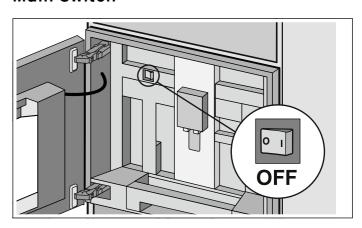
The main switch is used to switch the appliance on and off.
