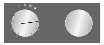
2 Use the > symbol to successively select the desired beverage, size, strength, temperature and coffee-milk ratio and use the rotary selector to save the settings.
