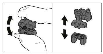
Separate the milk hoses, connecting element and milk tube.
