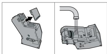
10 Remove the cover and clean the filter under running water.
