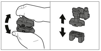
4 Separate the milk hoses, connecting element and milk tube.
