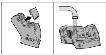
**10** Remove the cover and clean the filter under running water.
