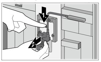
Detach the milk hose and dismantle the top and bottom sections of the beverage dispenser.
