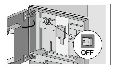
The main switch is used to switch the appliance on and off.
