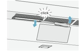
2 Remove the used odour filter and replace with a new odour filter.
