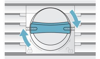
7 When installing a water filter: switch the water filter counter on.
