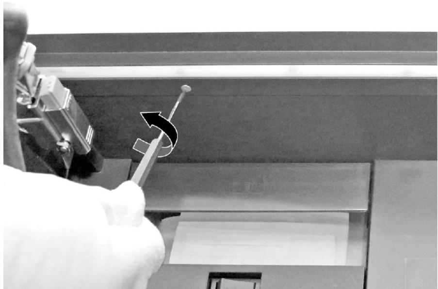
3. Press with the thumb from right to left hand side upwards until the glued panel is released.
