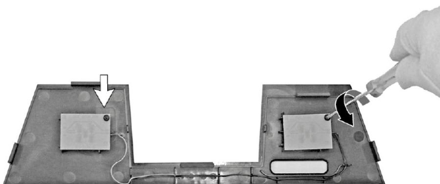
9. Pull out and remove LED light units.
