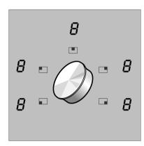
The twist knob is magnetic and is placed on the twist pad. The corresponding hotplate is activated by sliding the twist knob in the direction of the arrow. You can set the heat setting by turning the twist knob.
