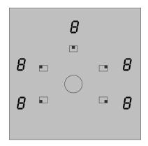
The twist pad is the area in which you select the hotplates with the twist knob and can set heat settings. The twist knob automatically centres itself in the twist pad.
