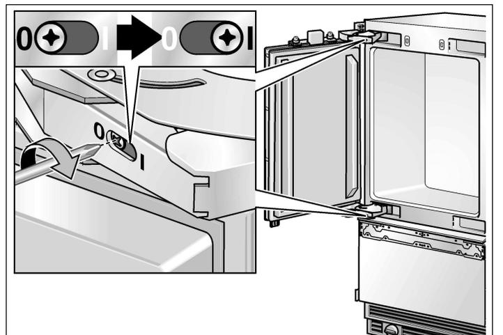
❑ Span the spring on the hinge. Tighten the screw from 0 to 1.
