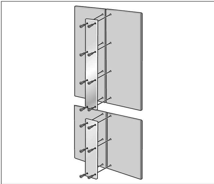
When attaching the metal strip to the furniture doors, observe the maximum possible length of the screws and the position of the drill holes. Always screw into the best load-bearing material of the furniture door.
