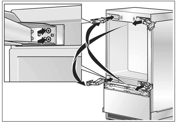
❑ Fix the hinges on the appliance. Change the hinges crosswise!
