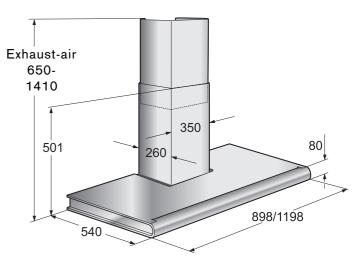
The exhaust air is discharged upwards through a ventilation shaft or directly through the outside wall into the open.
