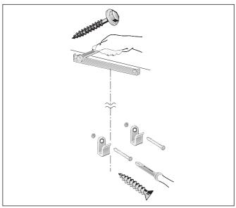
5 Screw on the upper and the two lower fixing brackets.
