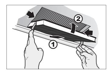
3 Insert the metal grease filters (see "Removing and inserting the metal grease filters").
