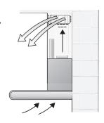
With activated carbon filter if exhaust-air mode is not possible.
