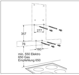
7 Remove the extractor hood. Drill the 4 lower 8 mm ø fixing holes and press in the wall plugs flush with the wall..
