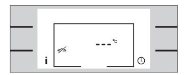
For your protection the appliance has a safety deactivation. The safety deactivation switches off the heat if the oven is left on for more than 12 hours without the controls being touched.
