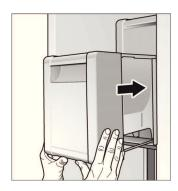
• If the container cannot be pushed all the way back, twist the screw conveyor in the container.
