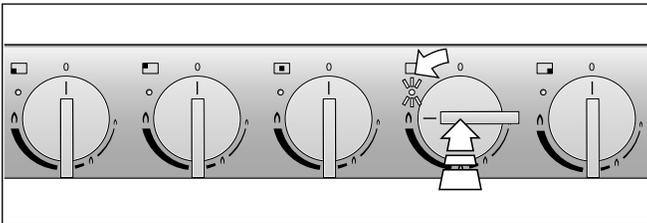
By slowly turning the control knob, the flame size can be steplessly adjusted between full and low flame.
