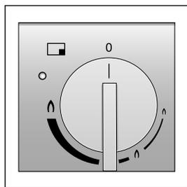
The markings on the control knob show which burner it is for and the setting from low to full flame. Setting is stepless.
