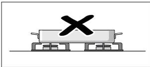
Never heat a cooking vessel (e.g. roasting tin, pan, cooking stone) with multiple burners. The resulting accumulation of heat causes damage to the appliance.
