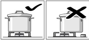
Place the cooking vessel in the center of the burner, otherwise it may tip over.
