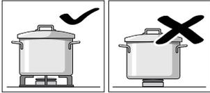
Place the pots on the pan supports, never directly onto the burners.
