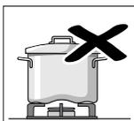
Don't use any deformed cooking vessels that don't stand solidly on the cooktop. The vessels could tip over.
