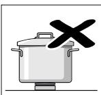
Place the pots or pans on the pan support, never directly on the burner.
