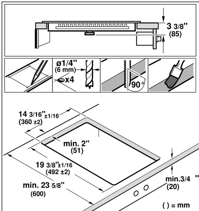
**Flush installation:** The appliance can be installed in the following temperature- and water-resistant countertops:
