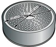
For good cooking results, the diameter of the cookware's ferromagnetic area should match the size of the hotplate. If cookware is not detected on a hotplate, try it on the next smaller hotplate down.
