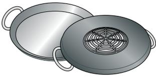
Cookware with aluminium on the base reduce the ferromagnetic zone, so less heat may be supplied or be difficult to detect.
