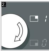
3 To change the power level: select the hotplate and change the power level desired using the Tipp control.
