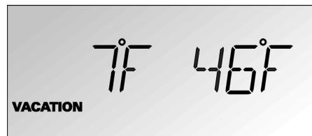
The **VACATION** symbol is displayed. Instead of the required temperature, the presetting temperature is displayed.
