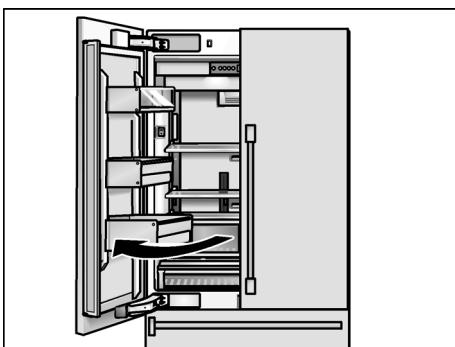
The 3-door variant allows for the left refrigerator compartment door to be opened without first having to open the right door.
