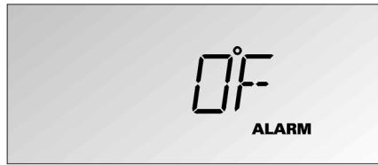
A temperature alarm is indicated by the required temperature flashing and the **ALARM** symbol coming on. A signal also sounds if the Tone function has been activated in Setup mode.
