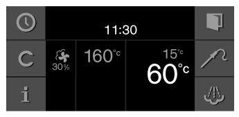
The appliance heats with the set heating mode. The current core temperature is displayed and, under it, the set core temperature. You can change the set core temperatur at any time.
