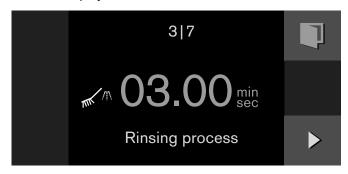
The descaling aid has ended. Delete the descaling hint in the display. Touch  $\checkmark$  to confirm.
