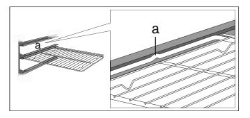
When pushing in the unperforated cooking container, make sure that the recess (a) is pointing to the side.
