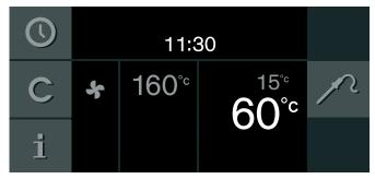
The appliance heats with the set heating mode. The current core temperature is displayed and, under it, the set core temperature. You can change the set core temperatur at any time.
