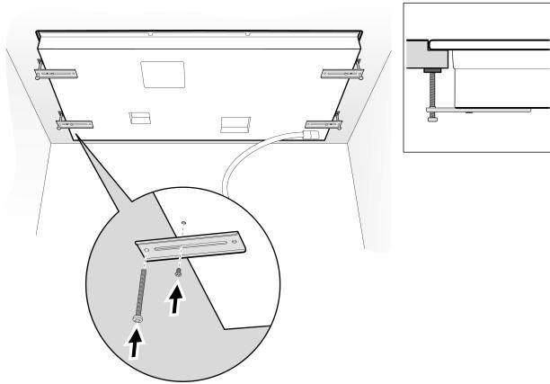
Not to let the glass to “drop” into place and that it needs to be supported along a broad area of the edges when “placing” the cooktop into the cutout.
