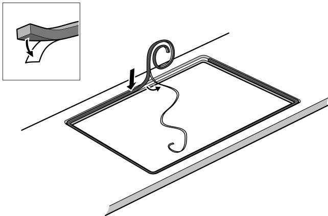
Attach the adhesive seal around the edge of the countertop (see diagram).
