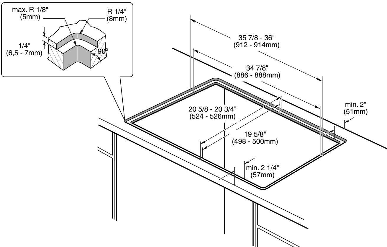
Solid surface countertops often require special installation. For example, heat reflective tape or rounded corners may be necessary. Contact the countertop manufacturer for instructions specific to your countertop.
