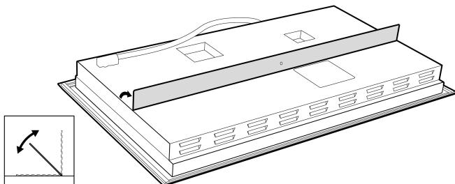
The heat shield will be able to rotate freely, as shown in the illustration.
