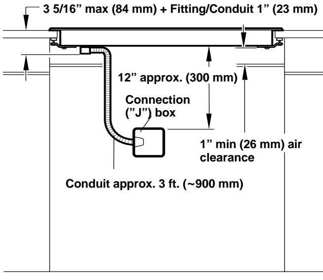
You can find the identification plate with the electrical specifications on the underside of the appliance. The junction box must be located within 3 feet (~900 mm) of the cooktop connection. It should be easily accessible for service purposes.
