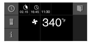
The appliance assumes a waiting mode. The operating mode, the temperature, the cooking time and the end of the cooking time appear in the display. The appliance starts at the calculated time and switches off automatically when the cooking time has elapsed.
