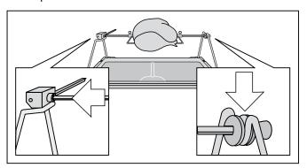
Insert the rotisserie spit in the lowest insertion level in the oven. The drive spindle must engage in the opening on the oven's rear wall.
