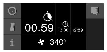
The appliance switches off after expiration of the cooking time. The  $\bigcirc$  pulsates and a signal sounds. It goes off prematurely if you touch the  $\checkmark$  symbol, open the appliance door or set the program selection to  $\mathbf{0}$ .
