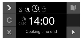
**3** Set the required cooking time end with the rotary selector.
