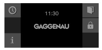
The child lock is activated. The standby screen appears. The  $\bigcirc$  appears at the top of the display.
