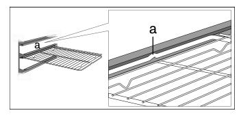
When pushing in the perforated cooking receptacle, make sure that the recess (a) points to the side.
