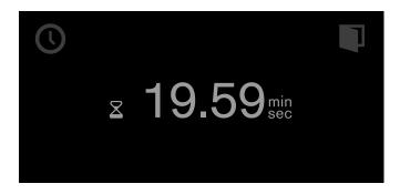
A signal sounds once the time has elapsed. The audible signal ceases if you touch the  $\checkmark$  symbol.
