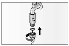
4. Carefully turn on the tap and check that the connection points are not leaking.
