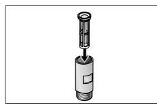
2. Place seal in the filter housing and connect to the tap (¾" threaded connection).
