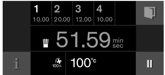
**Note:** You can change the temperature with the rotary selector while the recipe is running. This does not change the stored recipe.
