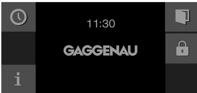
The child lock is activated. The standby screen appears. The
