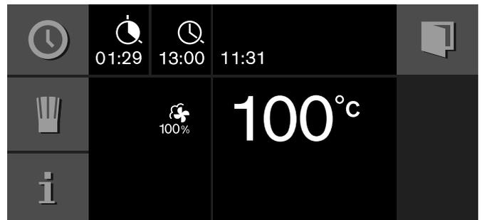
During the last minute of the cooking time the remaining time is displayed in an enlarged format.
