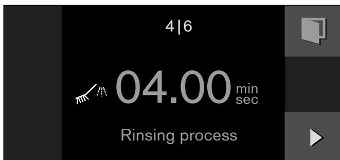
A signal sounds after 4 minutes. Touch
