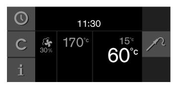
The appliance heats with the set heating mode. The current core temperature is displayed and, under it, the set core temperature.
