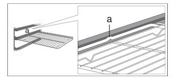
When pushing in the perforated cooking container, make sure that the recess (a) is pointing to the side.
