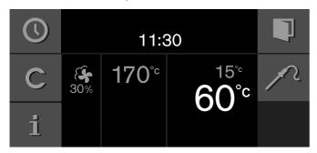
The appliance heats with the set heating mode. The current core temperature is displayed and, under it, the set core temperature.
