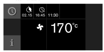
The appliance switches to standby. The operation mode, the temperature, the cooking time and the cooking time end are shown in the display. The appliance starts at the calculated time and switches off automatically when the cooking time has elapsed.
