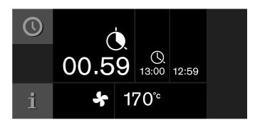
Once the cooking time has elapsed, the appliance switches off. The symbol pulsates and a signal sounds. The signal stops when you touch the symbol, open the appliance door, or set the function selector to 0.
