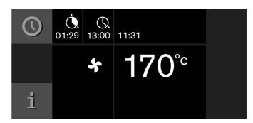
One minute before the cooking time ends, the cooking time that is counting down is enlarged in the display.
