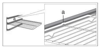
When pushing in the perforated cooking container, make sure that the recess (a) is pointing to the side.
