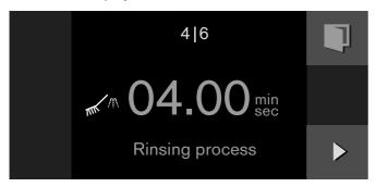
An signal sounds after 4 minutes. Confirm with  $\checkmark$ . Dry the cooking compartment with a soft cloth and dry fully with the drying programme.
