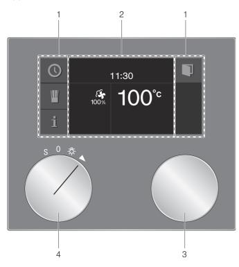
Operating controls on the lower side of the appliance
