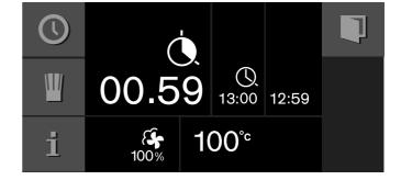
The appliance switches off after the cooking time has elapsed. The  $\bigcirc$  symbol flashes and a signal sounds. The signal stops when you touch the  $\checkmark$  symbol, open the appliance door, or switch the function selector to  $\bigcirc$ .
