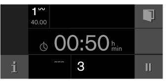
The appliance goes into standby mode. The display shows the operating mode, the grill setting, the cooking time and the remaining time until the start. The appliance starts at the calculated time and automatically switches off once the cooking time has elapsed.
